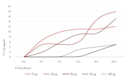
Notes: Five different viscosity oils ranging from 9 to 69 cp have been tested. Sample size: 1,000 capsules filled at 60% of body volume. Tested performed before banding operations.
