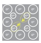
The removal of oxgen atom causes change of ratio of titanium atom to oxygen atom. This change of ratio induces the color change of titanium dioxide from white to grey.
