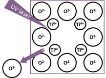
The ratio of titanium dioxide(Ti) to oxgen(O) in titanium dioxide is 1:2. UV laser is irradiated on the titanium dioxide then oxgen atom is removed.
