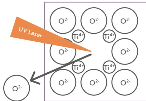
2 The removal of the oxygen atom causes a change of ratio of titanium atoms to oxygen atoms. This change of ratio induces the color change of titanium dioxide from white to grey.
