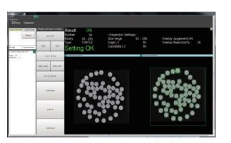
Printing is made easy with the use of a specialized camera detection system. Each product is recognized by its size, shape and location eliminating the possibility of print errors. The LIS-Labo can be used with various shapes and sizes of tablets and/or capsules. The camera detection system is easily viewed on a full color monitor screen. Up to 128 pieces/tray can be printed at one time while placed randomly in the easy to use product collection tray.
