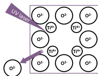
The ratio of titanium dioxide(Ti) to oxygen(O) in titanium dioxide is 1:2. UV laser is irradiated on the titanium dioxide then oxygen atom is removed.
