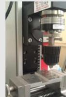
Figure 2. The Zwick materials testing machine with a capsule held in a bushing for puncture
