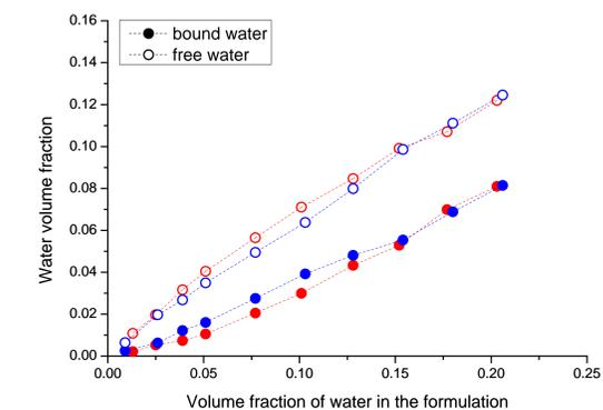
Moreover, the bound and free water fractions in the formulations could be differentiated with TD-NMR. This approach permits quantification of the relevant water fraction in the formulation that is directly available to interact with the capsule shell.
