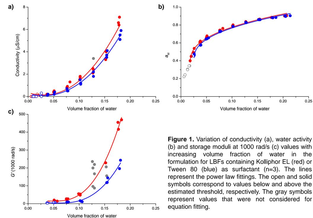
The results were modeled according to percolation theory and thresholds were identified for the formation of continuous water channels ( $\phi_{wc} \sim 0.02-0.06$ ). Thresholds were found to vary slightly depending on the physical property studied and they were slightly lower for the system containing Kolliphor EL. A new theoretical model for water activity based on percolation theory was also successfully introduced.
